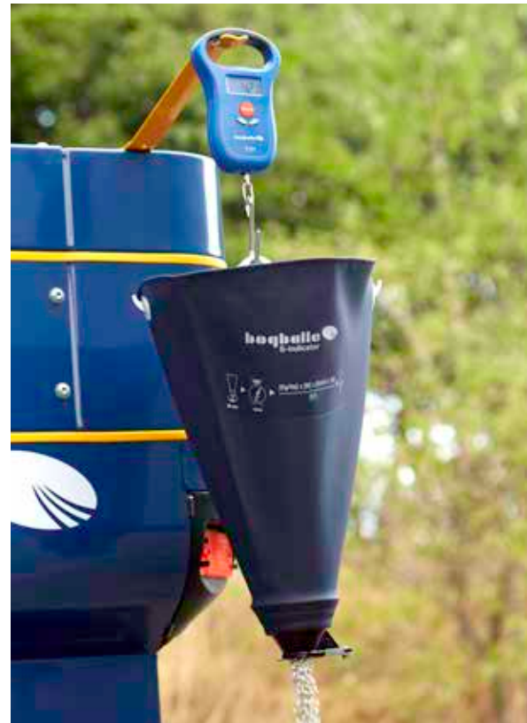
The S-indicator is easy to use and a complete flow test of a specific fertiliser is carried out in a few minutes.
