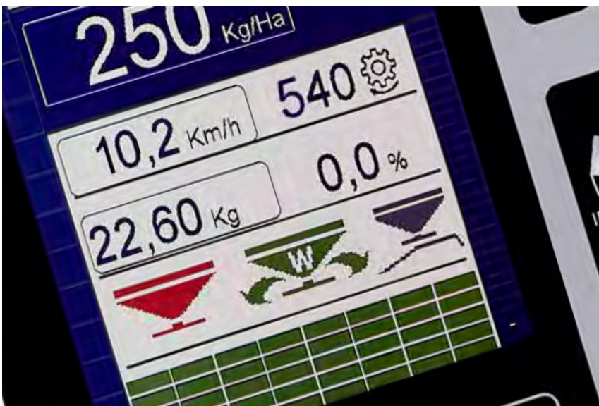
Spreaders fitted with weighing technique are automatically calibrated on the move, so there is no need for a manual flow test.
