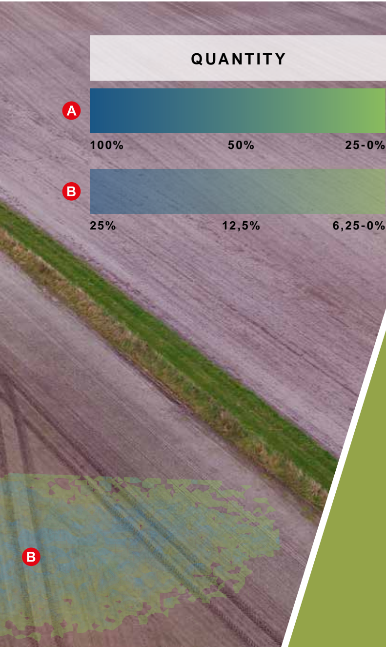
2D AND 3D MEASURING of Section Control Standard spread pattern with 40 sections open
