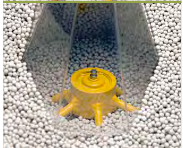
The free wheeling agitator keeps a constant flow of fertiliser by a gentle and eccentric rotation.
